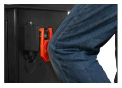
To turn the power off, simply bump or press the large red stop sign paddle.
